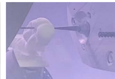
The design for the molar is sent to the CEREC Primemill where the block and the milling burrs are ready to make a crown come to life. The large burrs mill in parallel while the crown form becomes visible. It almost appears like the crown is being released free of the confinements of the zirconia block! To finish up all of the fine detail, the two small burrs take over. Being so small and sharp, these burrs can make very detailed tertiary anatomy. The entire time for milling was 4:22.
